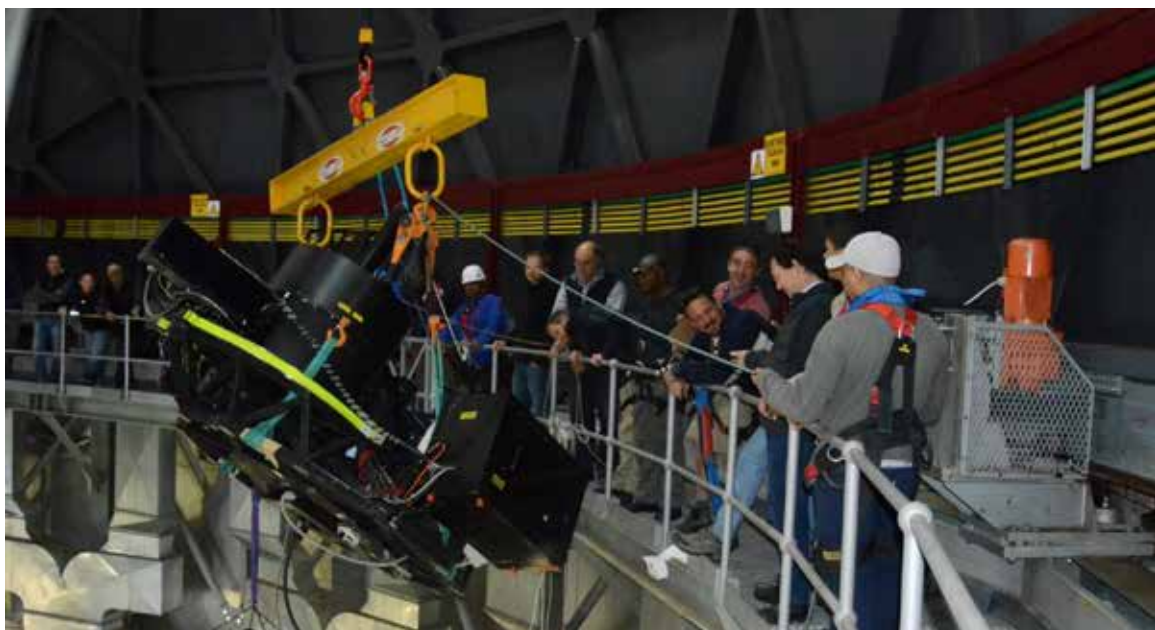
The RSS, with the new guider on-board, is being lifted to the tracker for re-installment.
