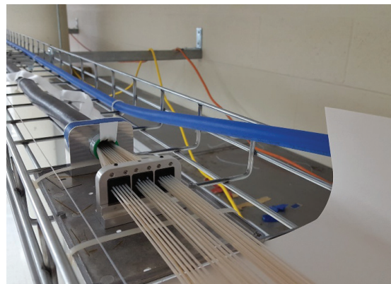
An 8-metre long prototype fibre cable has been constructed to test fabrication techniques and verify performance as a function of different environmental factors. Each individual optical fibre is slid inside a Teflon tube for protection and each of those tubes is held by a shear clamp at the ends of the cable (pictured here).
