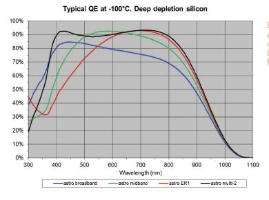
Quantum efficiency curves for the various coating options available for a deep depletion  $6K \times 6K$  device from CCD vendor e2v. The "Astro Multi-2" coating (black curve) would be the most suitable for the new RSS detector, as well as for the MaxE system.
