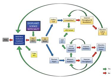
Flow chart describing the process of investigating the suitability of the HRS for exoplanet science. LFC = laser frequency comb and PFS = Planet Finder Spectrograph (on the 6.5-m Magellan II telescope).
