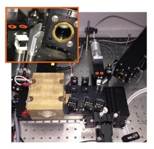
The high-stability bench showing the beige lodine Cell housing on the left, and the black translation stage (that moves horizontally) configured to direct arc light from the ThAr lamp (top right) into both HS-mode fibres (labelled P and D in orange, see inset) for the ThAr stability tests.
