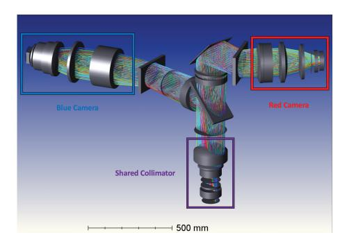
Optical layout for the new concept for the MaxE project: the addition of a red arm for the RSS, thus converting the instrument into a two-channel spectrograph.
