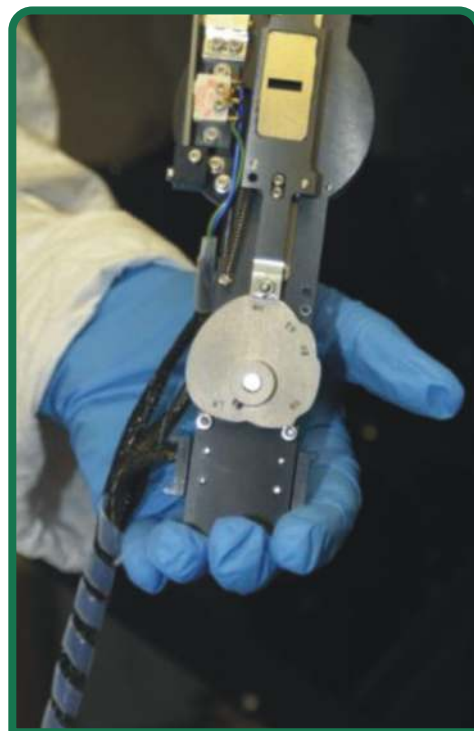
Preparing to open the HRS vacuum tank, after dismantling the grey Styrostone thermal enclosure (left), and the HRS mode selector assembly that needed attention, seen here after being removed from the optical bench (right).
