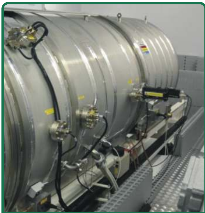
Preparing to open the HRS vacuum tank, after dismantling the grey Styrostone thermal enclosure (left), and the HRS mode selector assembly that needed attention, seen here after being removed from the optical bench (right).
