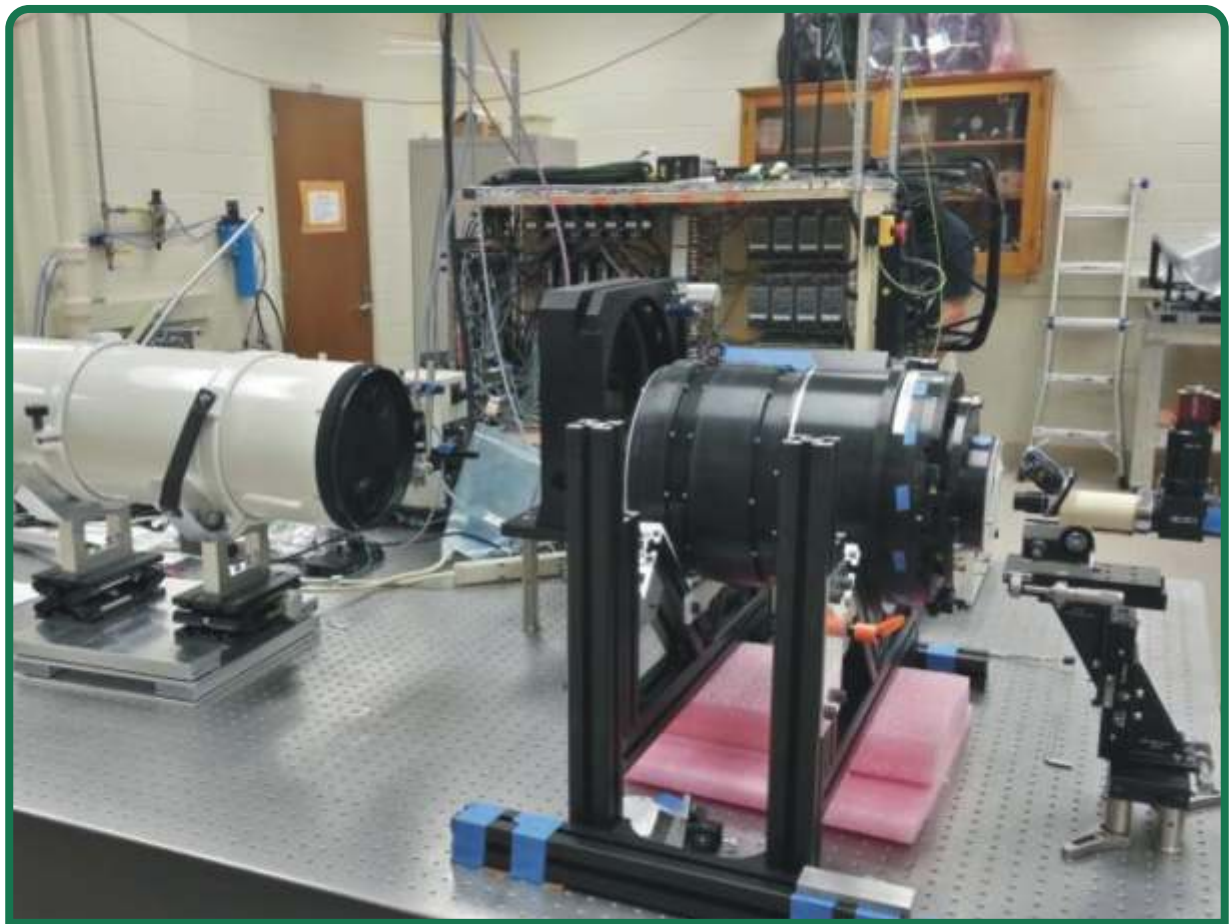
The new RSS-NIR camera test configuration with a fibre inspection camera
