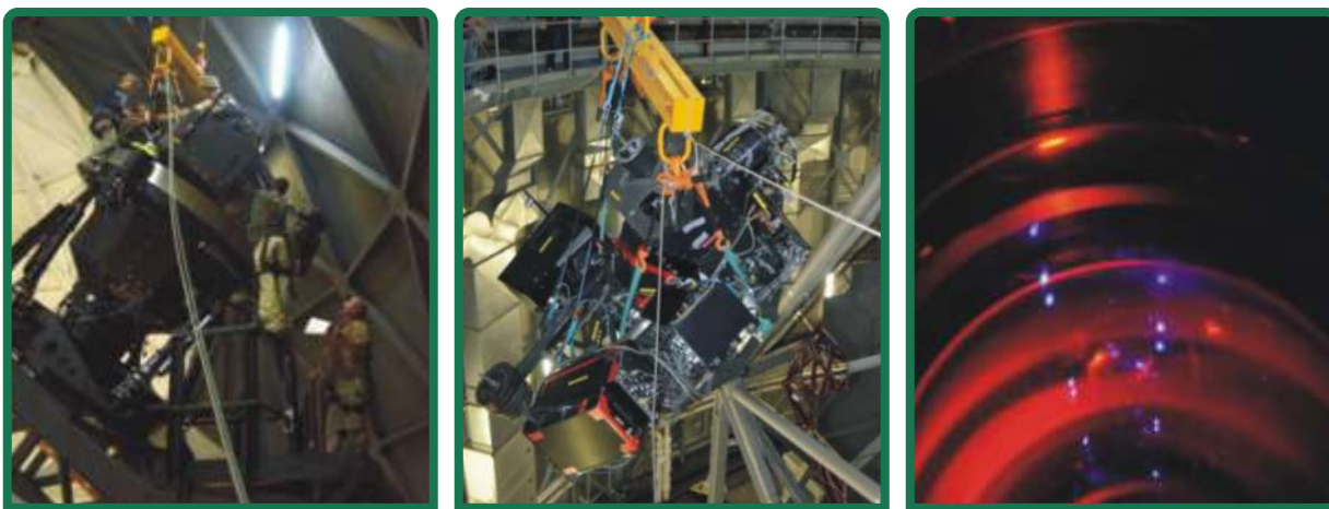
RSS being removed from the tracker (left), and lowered to the ground with the dome crane (centre). Red light illuminating the collimator lenses while a blue laser was set up to measure the throughput of the optics (right).
