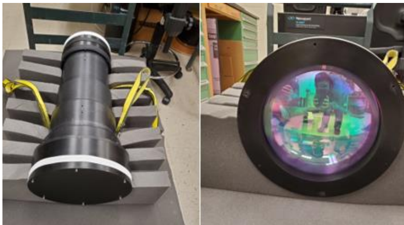
Above: NIR collimator barrel (left) and last optical surface (right).
