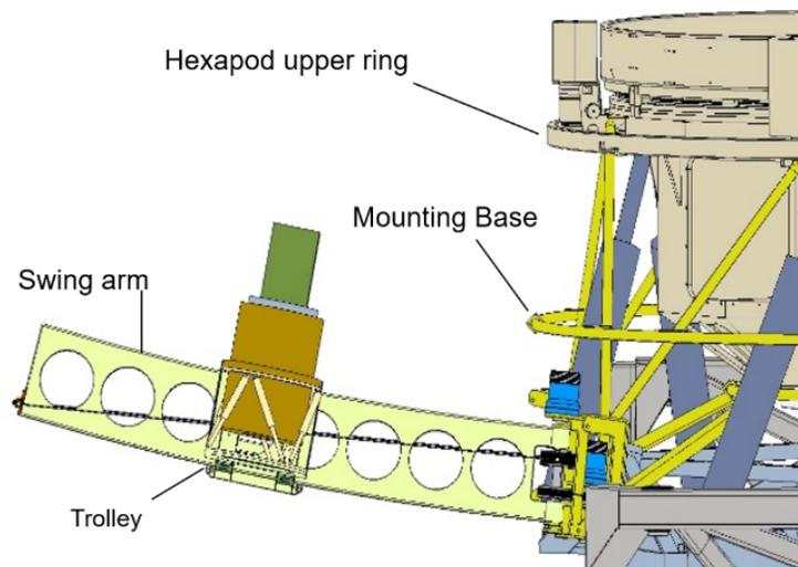
**Fig. 3:** The swing arm positioner (cable and drum drives in blue).
