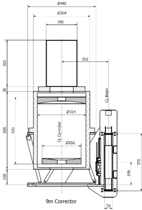
Fig. 9: Sectional view of the MSAC, swing arm, and trolley.
