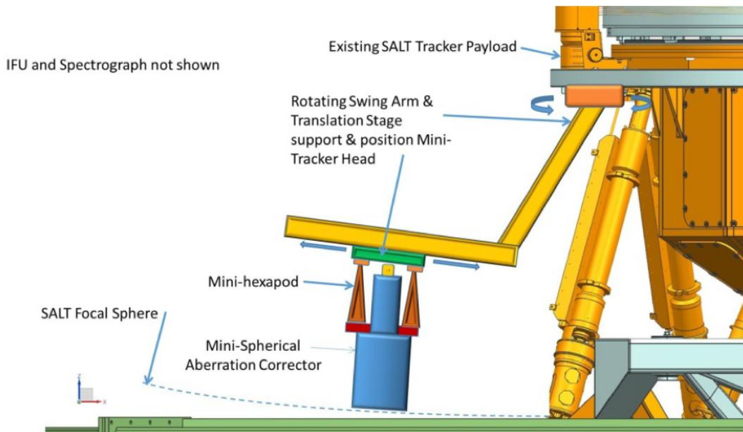
Figure 6. Concept PMRA - Payload-mounted Robot Arm, Side View.
