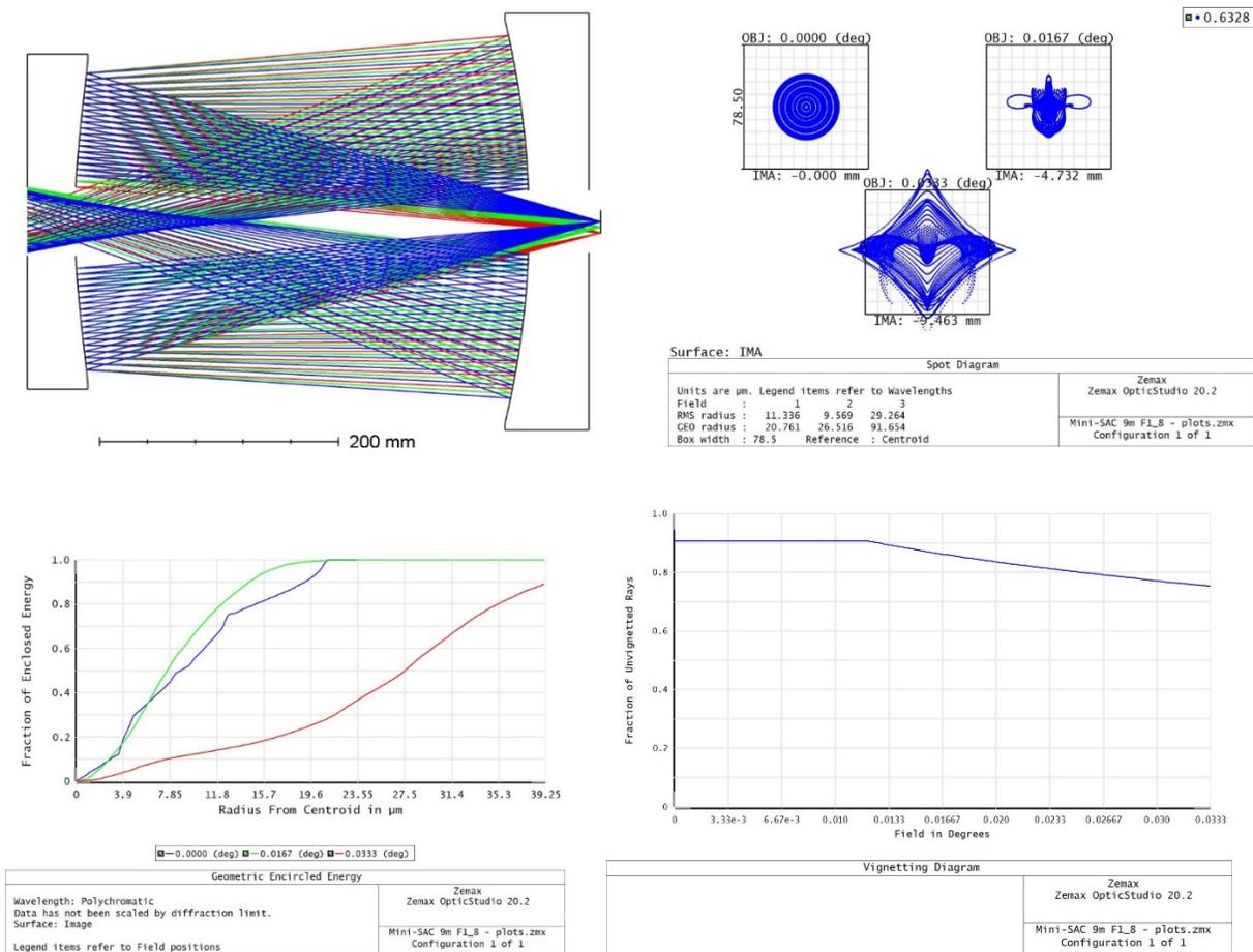
**Fig. 8:** The optical layout, spot diagrams, encircled energy and vignetting curves for the 9-m MSAC.
