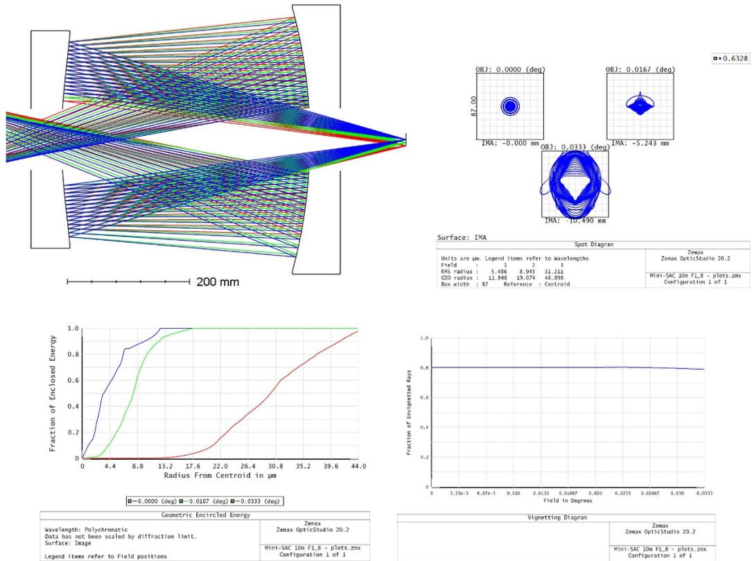
Fig. 10: The optical layout, spot diagrams, encircled energy and vignetting curves for the 10-m MSAC.
