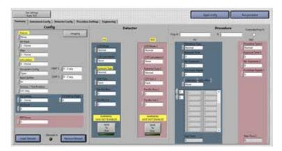
The new "Summary" tab for RSS Dual. A yellow background indicates differences between the current instrument settings and the fields displayed on the HMI.
