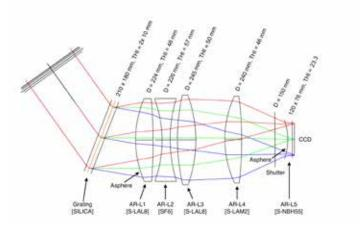
Figure 1: Optical layout of the Red collimator doublet (left) and camera (right).
