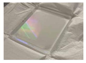
The new 700 I/mm VPH grating for the RSS being unwrapped in the lab.
