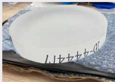
The 250 mm diameter x 52 mm thick S-LAL8 blank for AR_L3.
