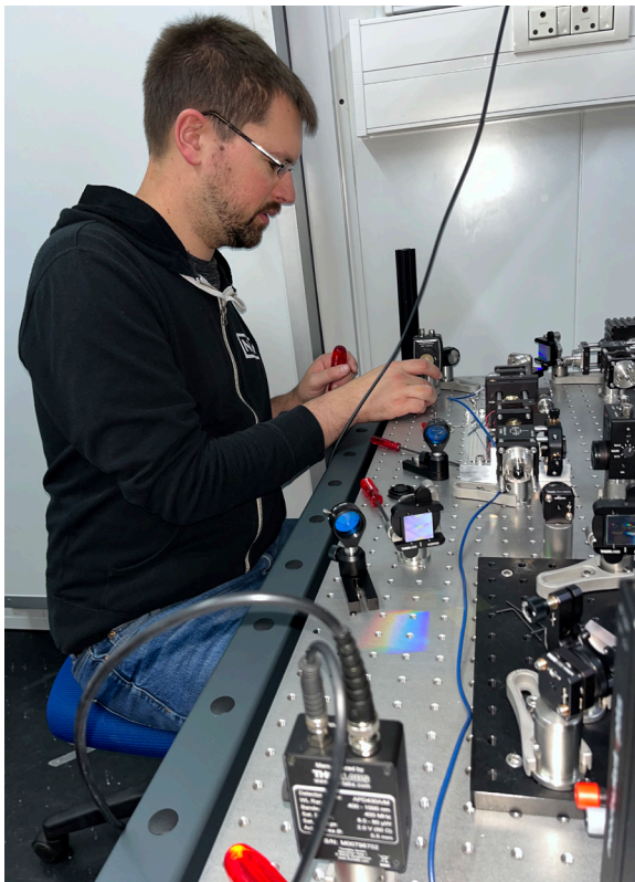
Richard McCracken from Heriot-Watt University aligning optical elements on the LFC bench.
