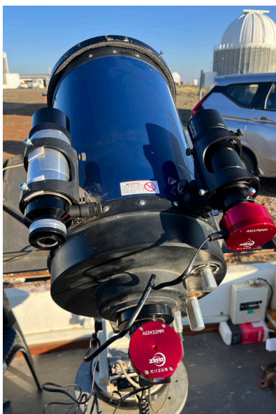
The telescope with the new seeing camera at the bottom and the new acquisition camera to the right (both in red).
