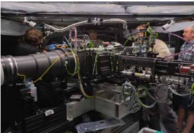
Left to right: Etienne Simon (SALT), Nico van der Merwe (SALT), Michael Smith (UW), and Eben Wiid (SALT) removing the dewar for installation of a new filter during the November servicing mission.
