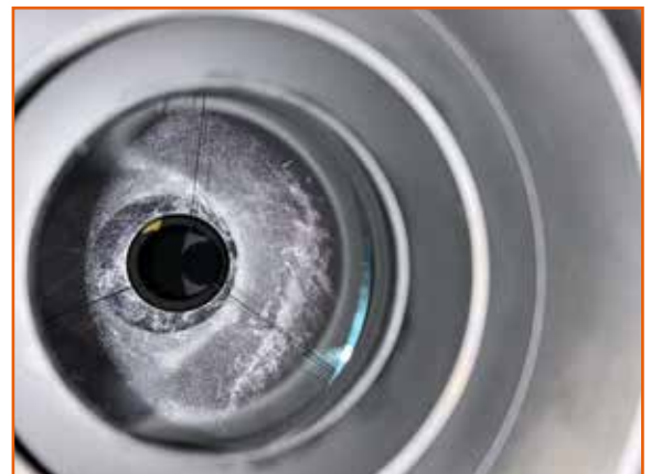
The M2 mirror showing the degradation in the coating.
